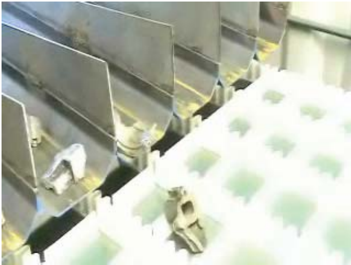
Figure 4: QXR-M multi-channel feeder with pocket conveyor belt, for high-speed singulation of materials.
