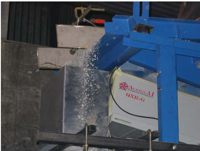
Figure 1: Austin AI's QXR-G, In-Line Cullet Inspection System
